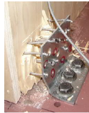
Fig.5: Typical responses of wooden wall panels exposed to combined vertical and horizontal load.
